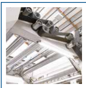
4 Driven rolls through reinforced belts or individual direct motors
