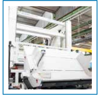
10 Automatic reels unloading with specific solution for narrow reels
