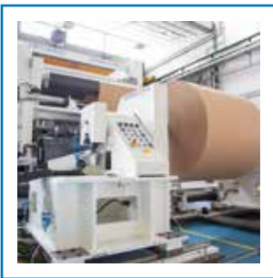
1 Shaftless unwinder (tambour execution available)
