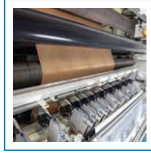
6 Automatic knife positioning
