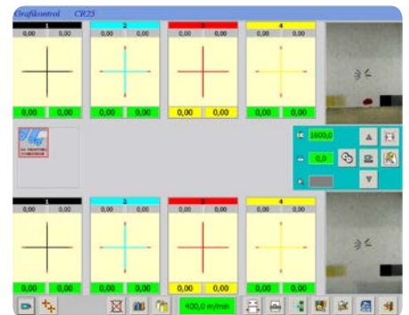
MAIN OPERATOR SCREEN, COMMERCIAL PRESS CONFIGURATION
