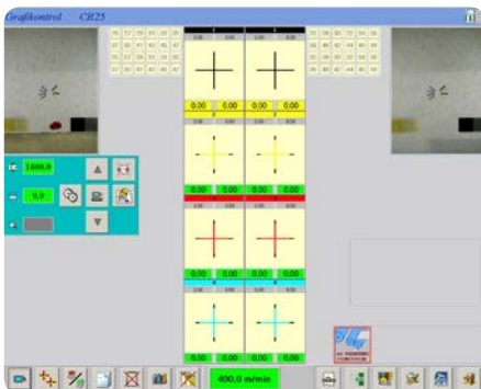
MAIN OPERATOR SCREEN, NEWSPAPER PRESS CONFIGURATION
