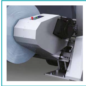
2 Unwind and rewind traverse movement is initiated by an electric drive concept
