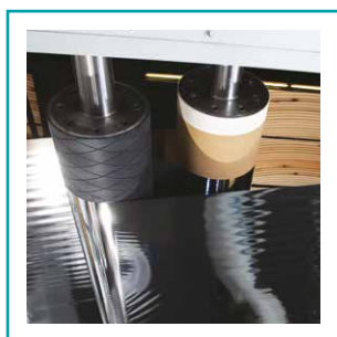
6 S-roller group with high wrap-around angle for optimal web tension separation
