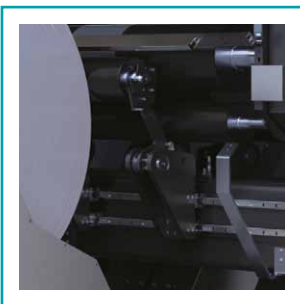
9 Easy and fast exchangeable contact rollers, no tools needed
