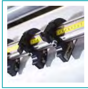
5 Blade oscillation function for razors slitting
